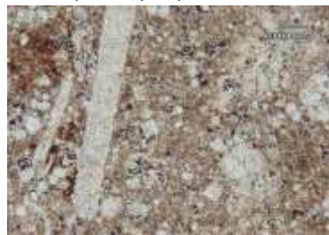
Micritic packstone with pyrite replacement of organic matter
