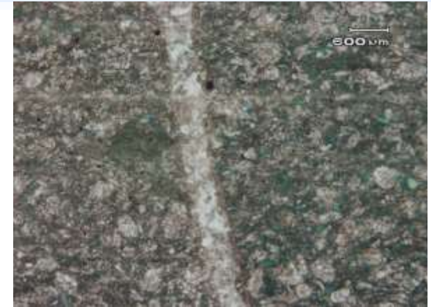
Fracture filled with sparry calcite due to Mesodiagenesis events.
